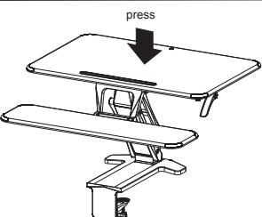
To prevent the tabletop bouncing and any property loss or personal injury, please press the handle to give the desktop downward force when you need to adjust the height while the object on the table is less than 6.6 lb.
