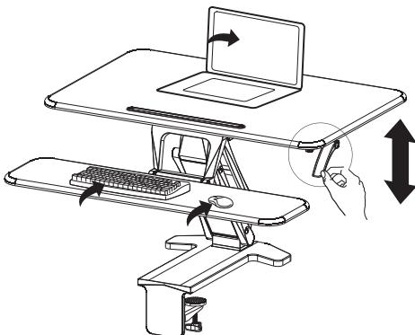
To operate the workstation, press the handle and raise or lower the top to desired height.
