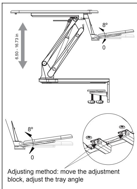
Adjusting method: move the adjustment block, adjust the tray angle
